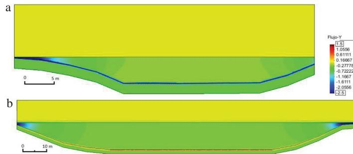
Fig. 3. Heat fluxes ( $\text{W}/\text{m}^2$ ). (a) in Santana dam; (b) in Esperanza dam.
