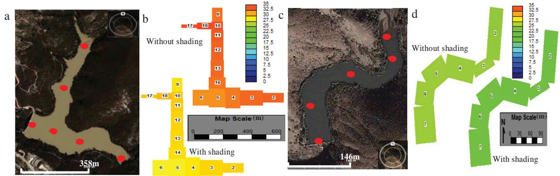
Fig. 2. (a) Esperanza dam; (b) W2 temperature simulation in Esperanza dam ( $^{\circ}\text{C}$ ); (c) Santana dam; (d) W2 temperature simulation in Santana dam ( $^{\circ}\text{C}$ ). Sample points are shown in red dots.
